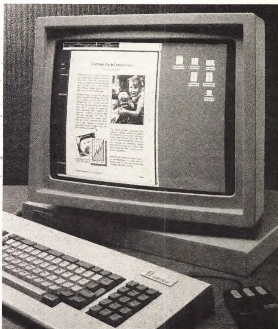
The Interleaf workstation. The screen shows the merged text and graphics, the icons or graphic menu, and the three-button mouse.
